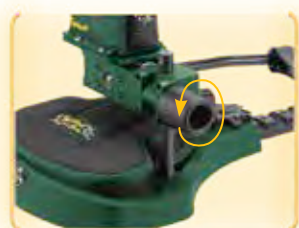
Fine and coarse elevation adjustment
